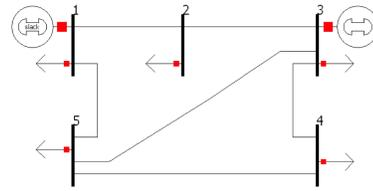
Figure 1: 5 Bus Power System Online Diagram [8]
